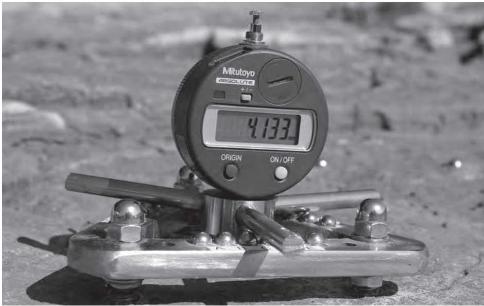
Fig. 2. The traversing micro erosion meter.
